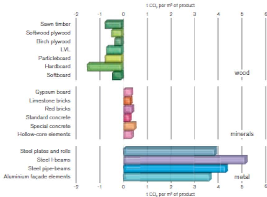
Figure 8 - Net CO<sub>2</sub> emissions of selected building materials during whole lifecycle
